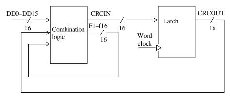
Figure 5.8 An example of generation of parallel CRC
